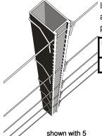
INSULATED TOP, GALV STEEL BASE. 940mm out of the ground. Install using a standard slide hammer. Notched every inch to provide reliable wire positioning. Wires held on using 'snap-on' or 'P-Type' wire clips.
