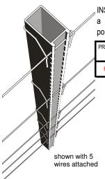
INSULATED TOP, GALV STEEL BASE. 1070mm out of the ground. Install using a standard slide hammer. Notched every inch to provide reliable wire positioning. Wires held on using 'snap-on' or 'P-Type' wire clips.
